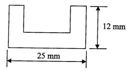
Take K=430 and n=0.19 for the work material. For Johnson's formula, assume a=0.8 and b=1.4. Calculate the ram force at stroke length= 400,300,200 & 100 mm and make an approximate plot. Use the shape factor formula as below:
