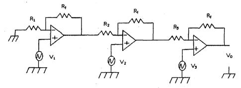
Where  $R_f$ =470k $\Omega$ ,  $R_1$ =4.3k $\Omega$ ,  $R_2$ =33k $\Omega$ ,  $R_3$ =33k $\Omega$ ,  $v_1$ =10 $\mu$ V,  $v_2$ =20 $\mu$ V, and  $v_3$ =40 $\mu$ V. (2+6+6=14)
