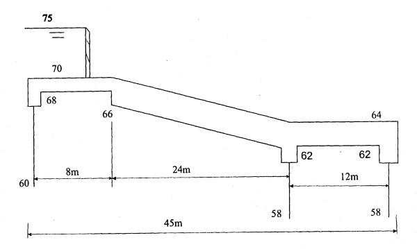
The profile of a weir is shown in the above figure. Find the corrected residual uplift pressures at the key points on upstream and intermediate pile using Khosla's theory. Use the table for slope correction.
